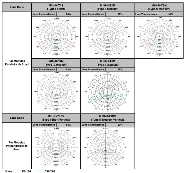
Installation guide: the arrow on the lens (parallel with C90/270) should be perpendicular to road and directs to road center.
